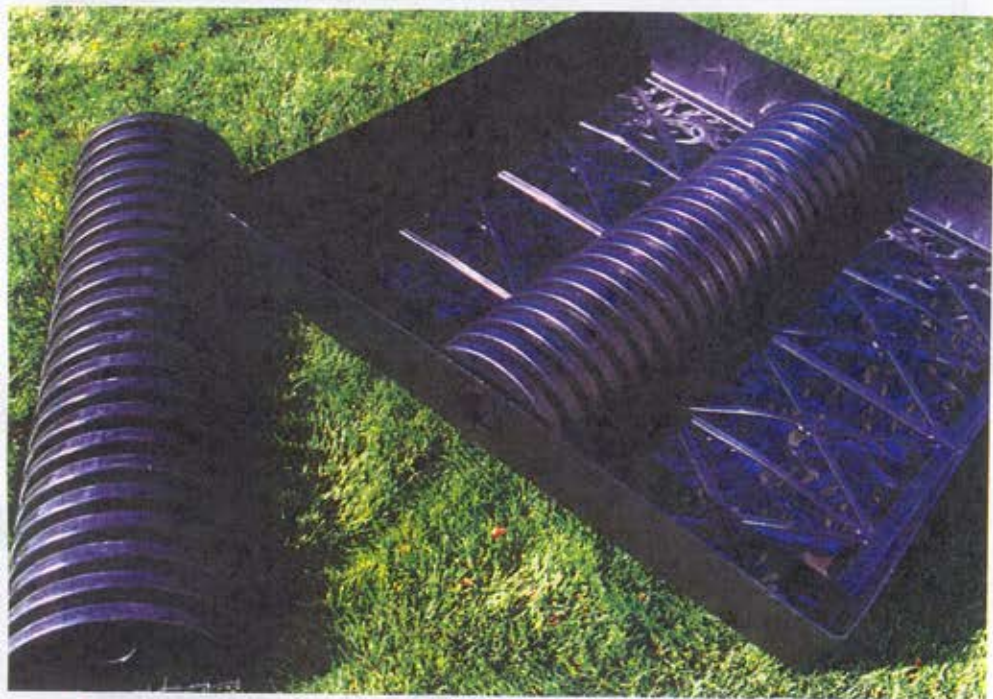
▲ The ECS underground pan prevents water loss to subsoil, while pipes control sand infiltration and direct water flow in a specific pattern through the chamber.
